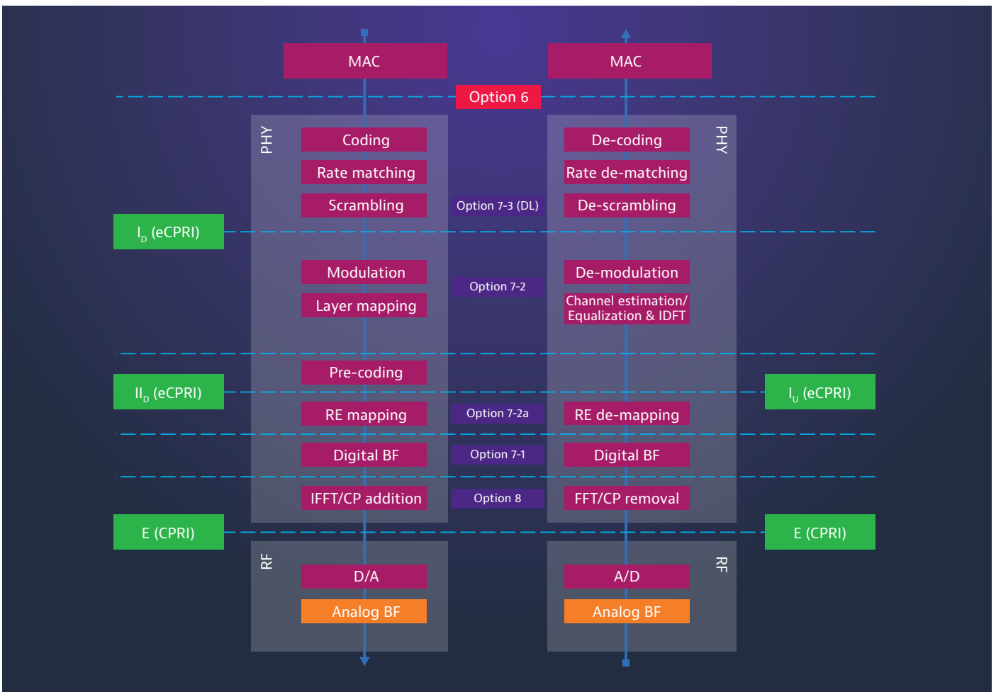
Figure 5: Functional Split in Phy (source: eCPRI specification)
